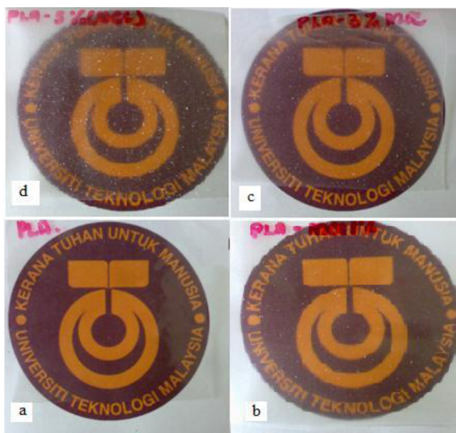
Fig. 6. Visual comparison of the transparency of (a) PLA and (b) PLA/MCC 1%, (c) PLA/MCC 3% and (d) PLA/MCC 5%.
